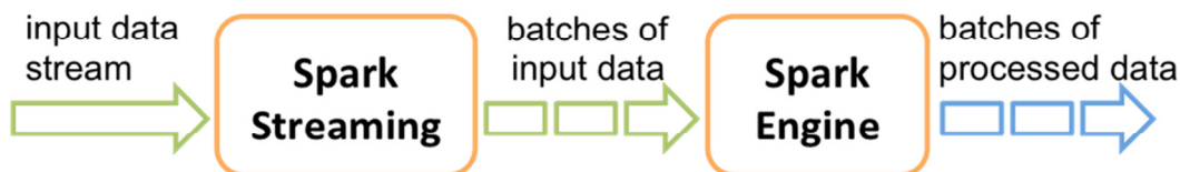
Figure 6.4 - D-Stream is a major concept in Spark Streaming
